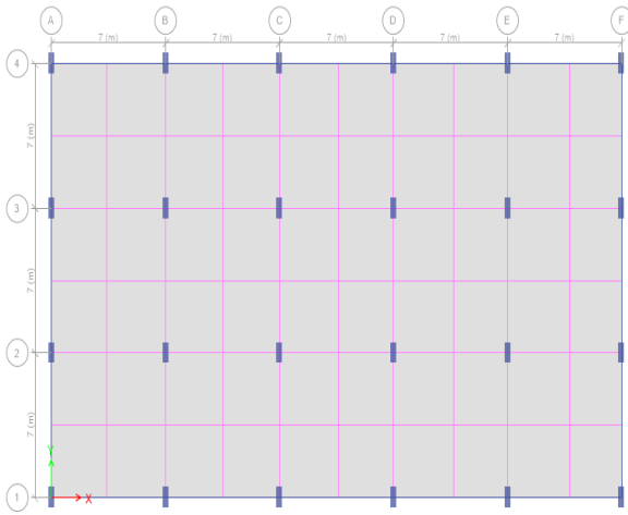
Flat Slab Without Drop.
